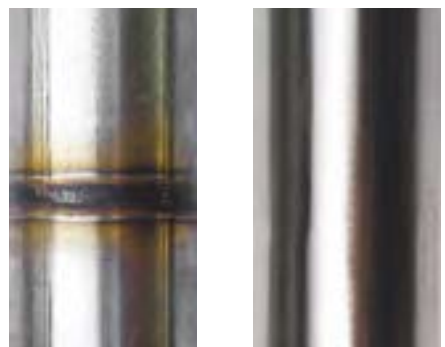
Cleaning and polishing of weldings on stainless steel tubes: before and after.
