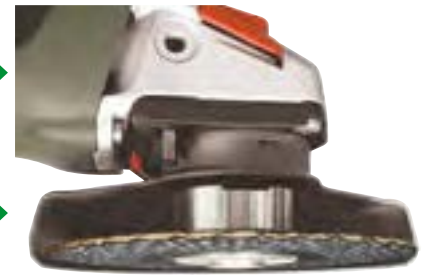
Flush mounting with the special GLOBE flanges.
